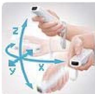
Figure 4. Wiimote motion axes.
